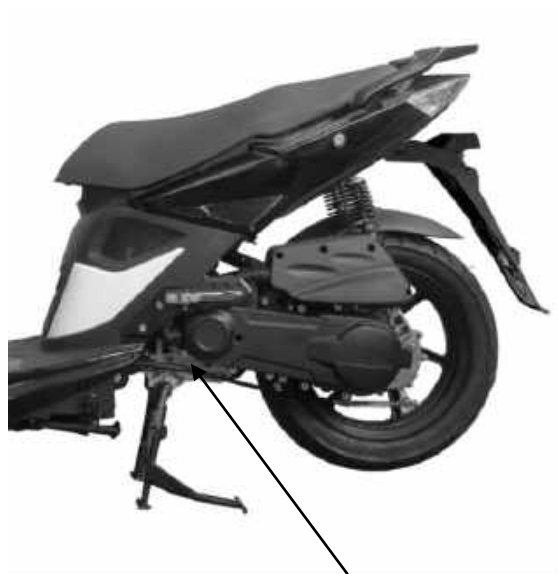
Location of Engine Serial Number
