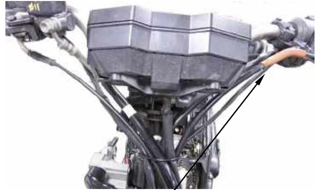
Stop Switch Wire
